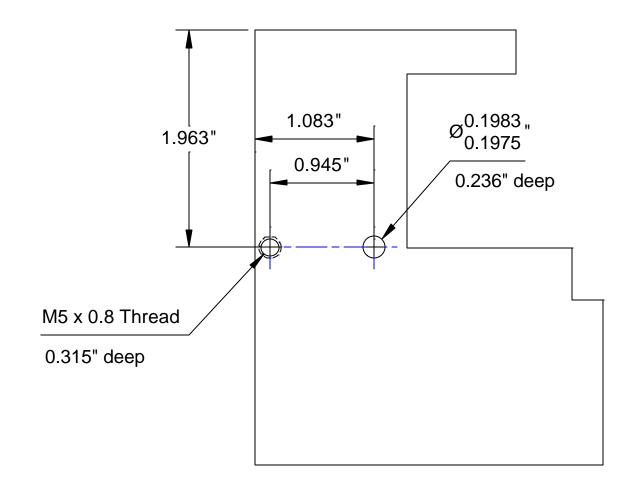
All dimensions are in mm Drawing is not to scale View is right side of carriage
