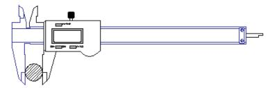
It's easy, but if you don't do it correctly the measurement will not be accurate. If the calipers are not straight (that is, perpendicular to the workpiece) the measurement will not be accurate. Likewise, if there is dirt on the jaws or the workpiece the measurement will not be accurate.
