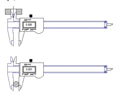
The caliper shows you how much material you need to remove, from either the shaft or the hole, to make them fit.
