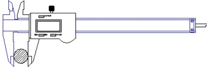
It's easy, but if you don't do it correctly the measurement will not be accurate. If the calipers are not straight (that is, perpendicular to the workpiece) the measurement will not be accurate. Likewise, if there is dirt on the jaws or the workpiece the measurement will not be accurate.
