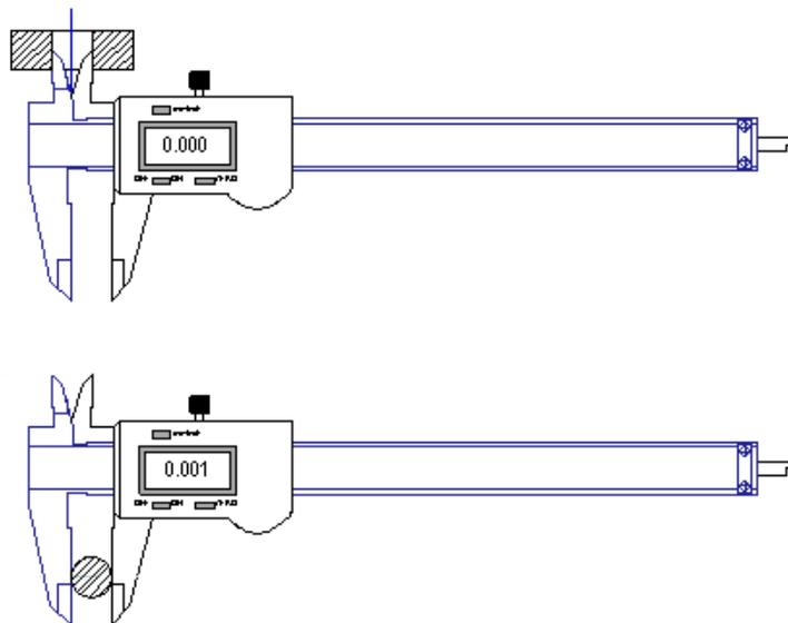
The caliper shows you how much material you need to remove, from either the shaft or the hole, to make them fit.
