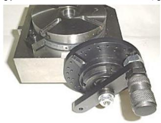
These instructions are for the LittleMachineShop.com 6" Precision Rotary Table part number 2326 and Dividing Plate Set part number 2328. (The photos in these instructions are of the 4" rotary table.)
