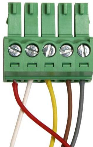
4. Insert each axis plug into the appropriate socket. Clamp the black-jacketed wire in the corresponding strain relief.
