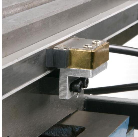
The drawing below shows the same thing along with the relationship of the mounting holes. As described later in this document, you might need to design and build a bracket and spacer to mount the magnetic read head as shown.
