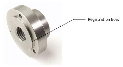
Lathe chuck adapters are made with the registration boss oversize so you can do the final machining on your lathe to fit your chuck. This ensures concentricity on your lathe. In some cases you will need to drill the chuck mounting holes also.
